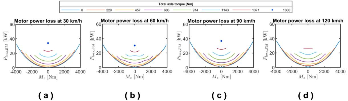
**Figure 2.** EM power loss as function of direct yaw moment for different total torque demand and vehicle speed of (a) 30 km/h, (b) 60 km/h, (c) 90 km/h and (d) 120 km/h.
