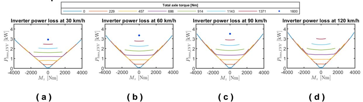
**Figure 3.** Inverter power losses at different vehicle speed (a) 30 km/h, (b) 60 km/h, (c) 90 km/h, (d) 120 km/h.
