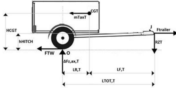
**Figure 17.** Longitudinal load transfer - free body diagram trailer.
