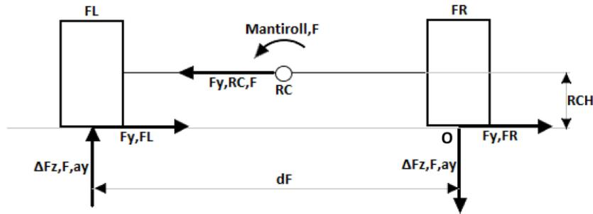
**Figure 20.** Lateral load transfer - free body diagram front axle towing vehicle.
