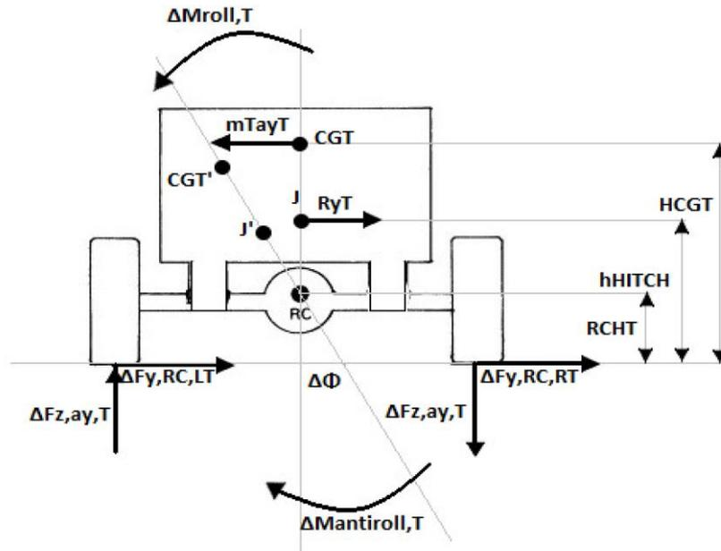
Figure 21. Lateral load transfer - free body diagram trailer rear view.
