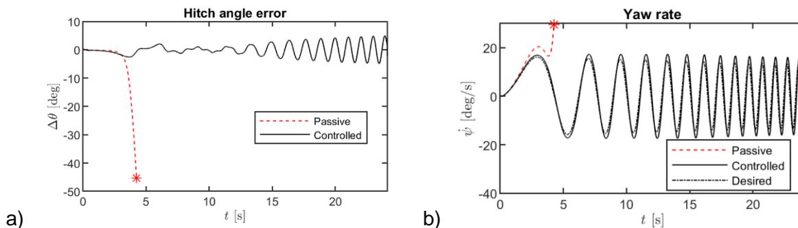
**Figure 30.** Hitch angle error (a) and yaw rate (b).
