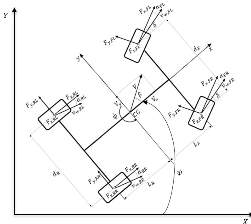
Figure 7. Four-wheel vehicle model.
