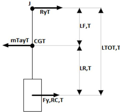
**Figure 24.** Lateral load transfer - free body diagram trailer top view.
