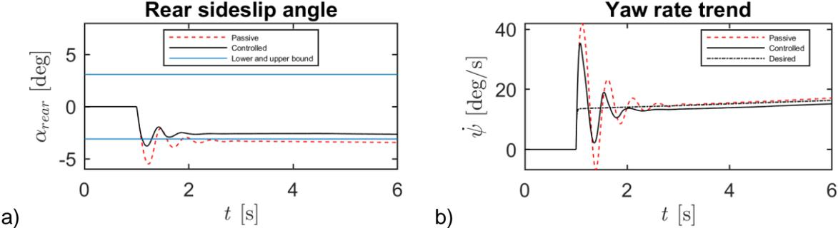
**Figure 12.** Step steer manoeuvre yaw rate tracking in emergency conditions at 120 km/h.
