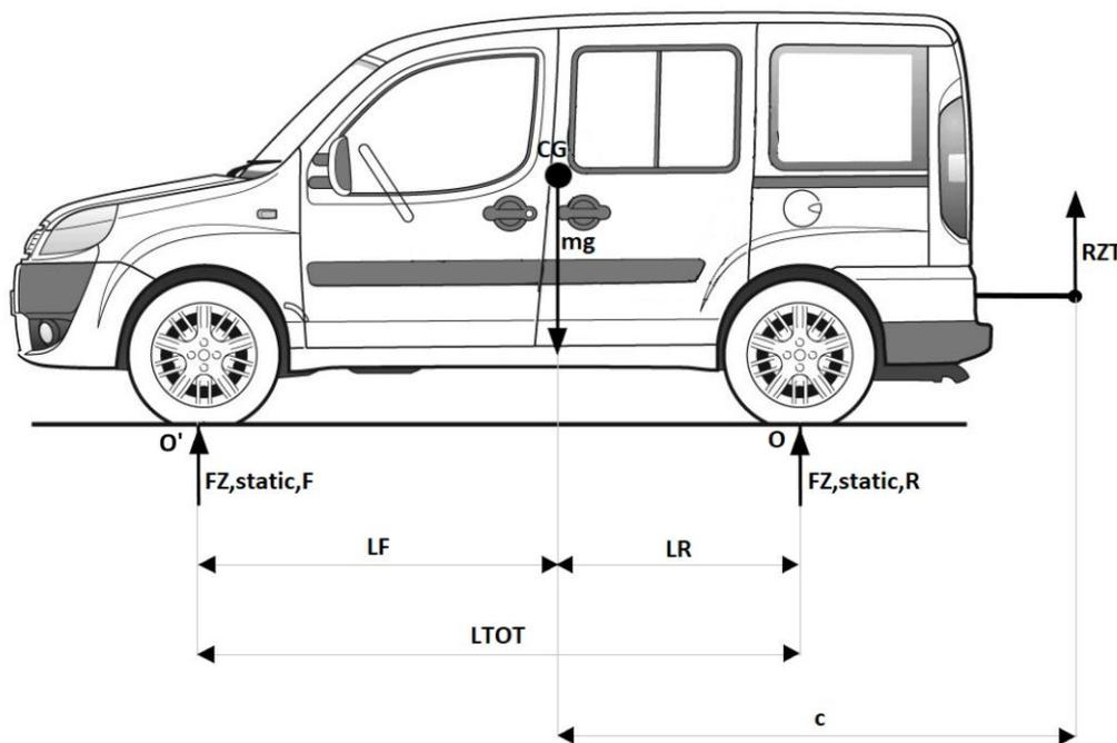
**Figure 14.** Static balance - free body diagram towing vehicle
