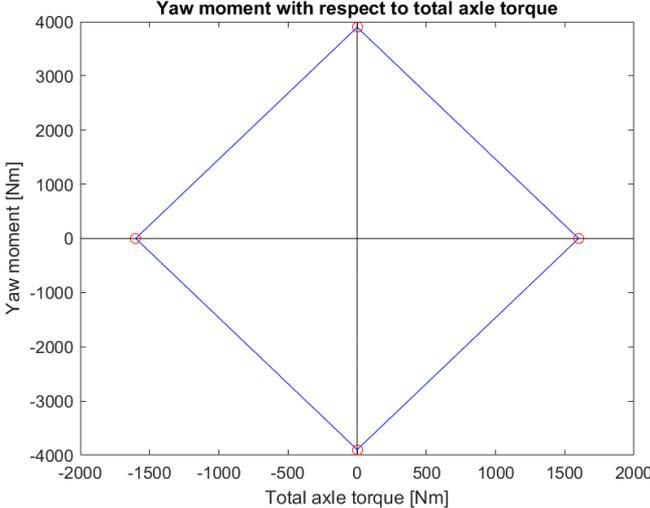
**Figure 6.** Yaw moment with respect to the total axle torque.
