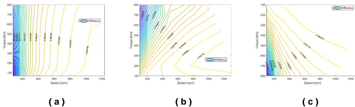
**Figure 1.** Experimentally measured (a) inverter efficiency, (b) motor efficiency in traction, (c) motor efficiency in regeneration.
