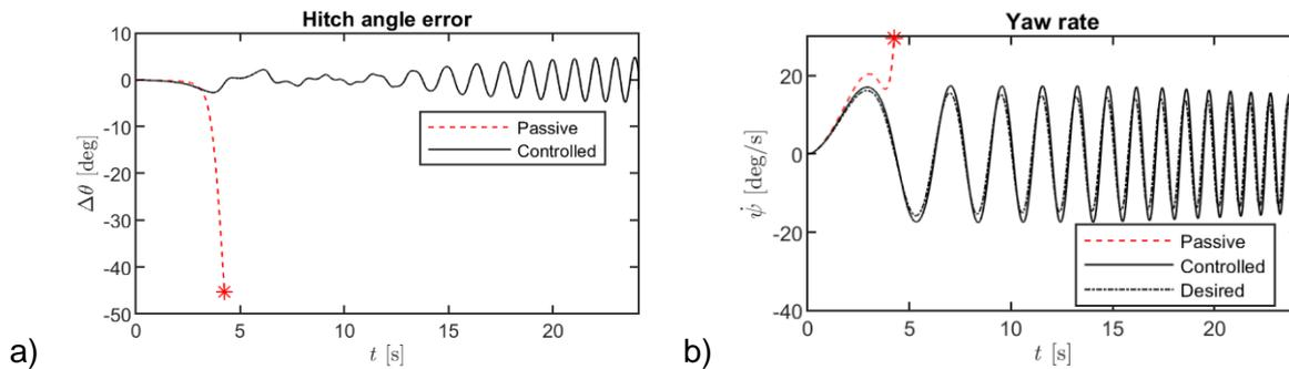
**Figure 29.** Hitch angle error (a) and yaw rate (b).
