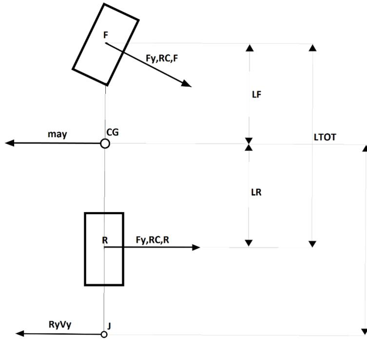
**Figure 25.** Lateral load transfer - free body diagram towing vehicle top view.
