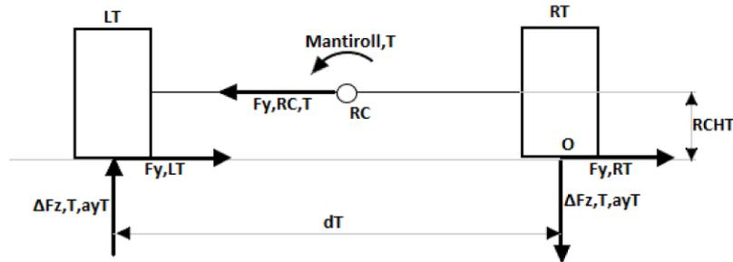
**Figure 23.** Lateral load transfer - free body diagram trailer axle.
