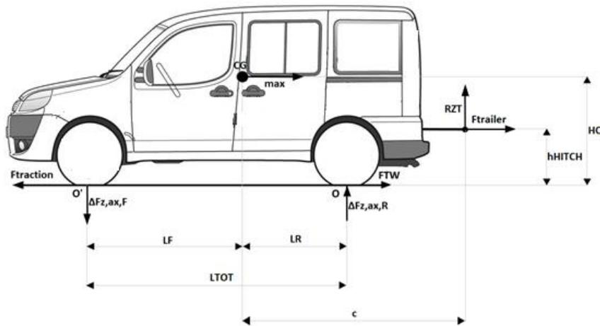
**Figure 16.** Longitudinal load transfer - free body diagram towing vehicle.
