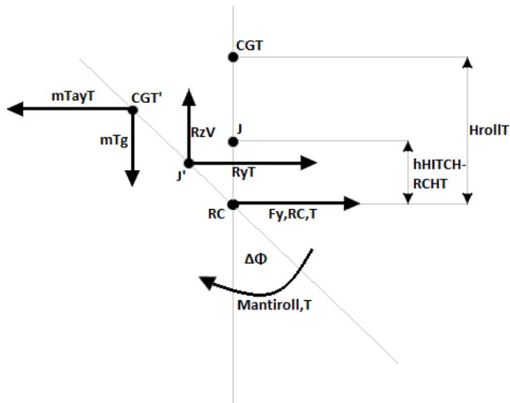
Figure 22. Lateral load transfer – trailer.
