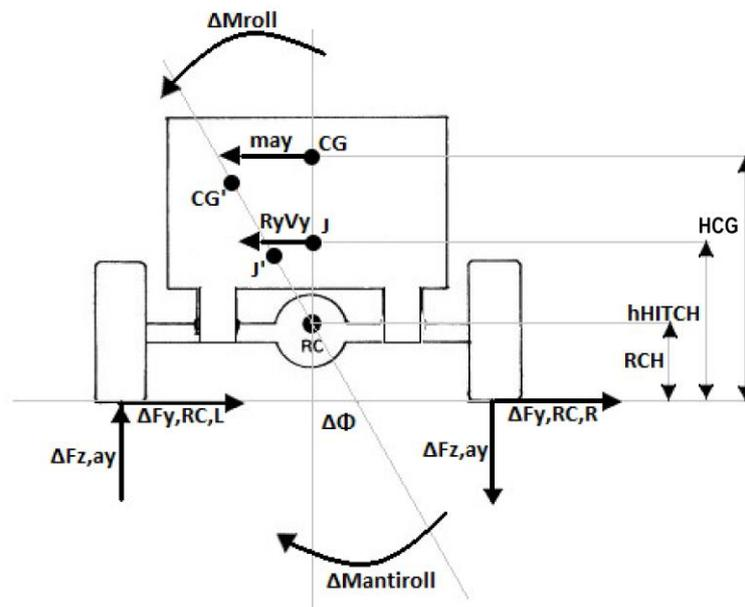
**Figure 18.** Lateral load transfer - free body diagram towing vehicle rear view.
