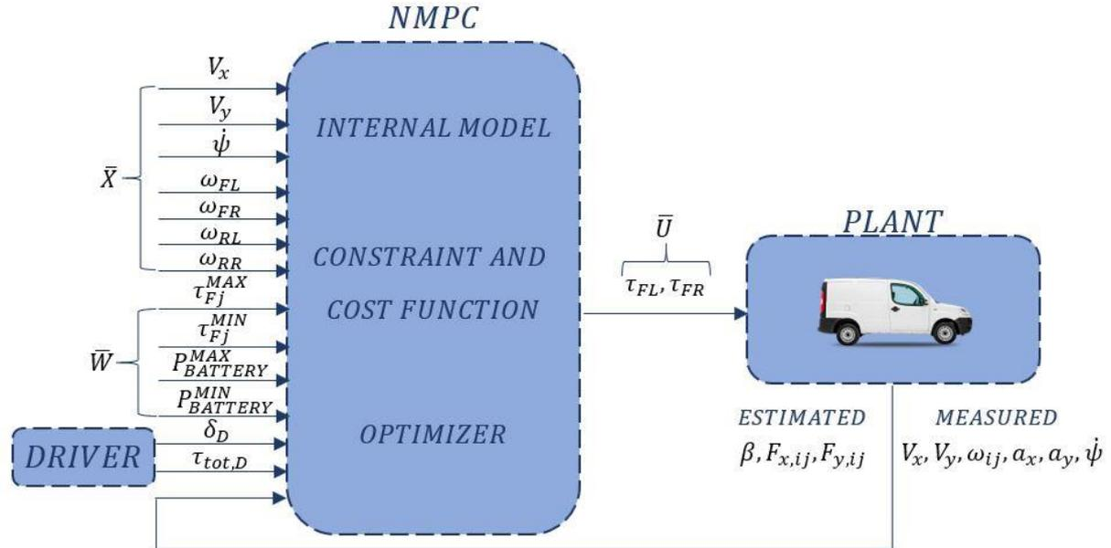
**Figure 9.** Schematic diagram for NMPC and plant – vehicle configuration.
