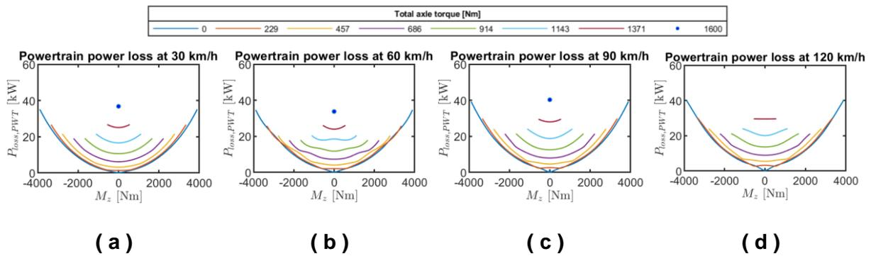
**Figure 4.** Powertrain power losses at different vehicle speed (a) 30 km/h, (b) 60 km/h, (c) 90 km/h, (d) 120 km/h.
