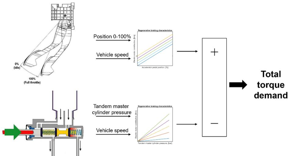
Figure 8. Regenerative braking system scheme
