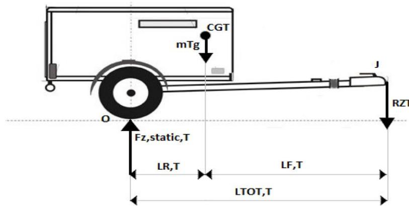
**Figure 15.** Static balance- free body diagram trailer.
