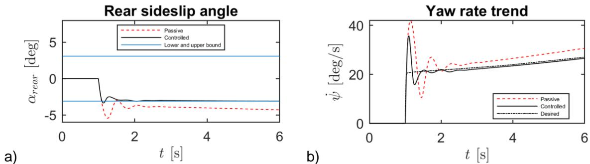
**Figure 11.** Step steer manoeuvre rear sideslip angle soft constrained at 80 km/h.
