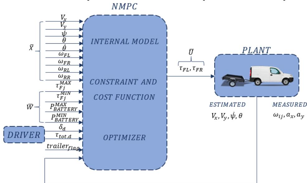
**Figure 26.** Schematic diagram for NMPC and plant – articulated vehicle configuration.
