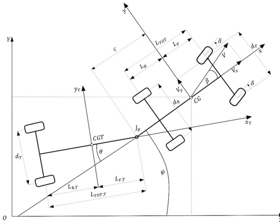
Figure 13. Articulated vehicle model.
