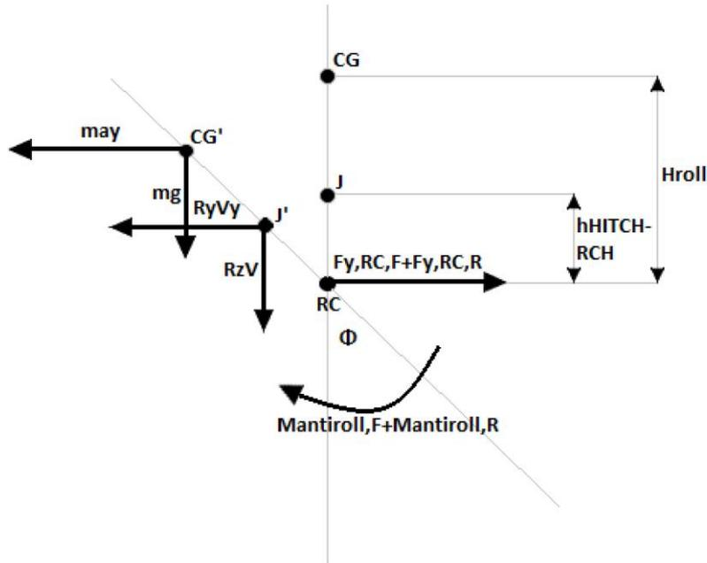
**Figure 19.** Lateral load transfer - towing vehicle.
