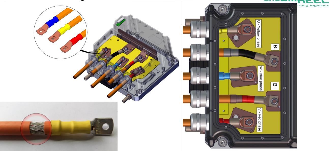
The cables and hoses shall be routed in such a way which ensures enough play for suspension movement. Sharp bending of the cables and hoses shall be avoided. If cables or hoses are in contact with sharp edges, additional protection must be added to avoid cable or hose damage.
